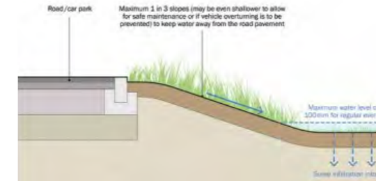
WATER FLOWS FROM SHALLOW SWALES ACTING AS EDGE DRAINS FOR THE ROAD SUB-BASE
