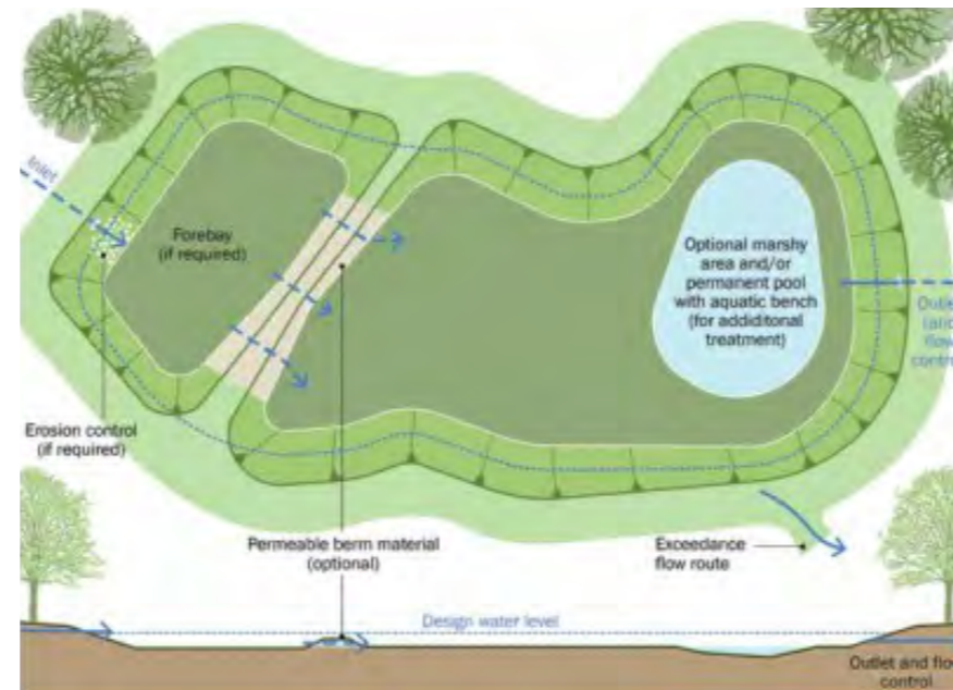
PLAN AND ELEVATION OF VEGETATED DETENTION BASIN
