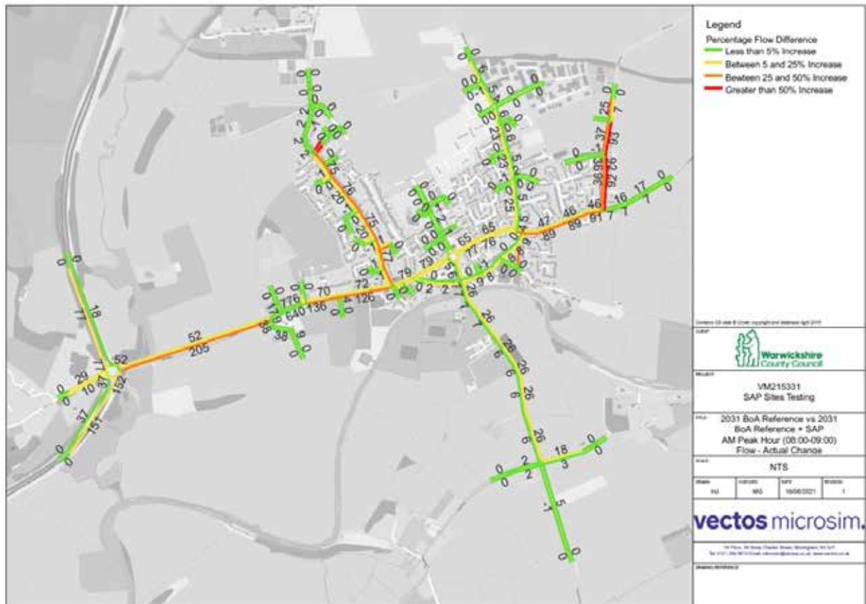
Figure 7 Flow Difference Plot – AM Peak Hour – Reference Case vs Reference + SAP Sites
