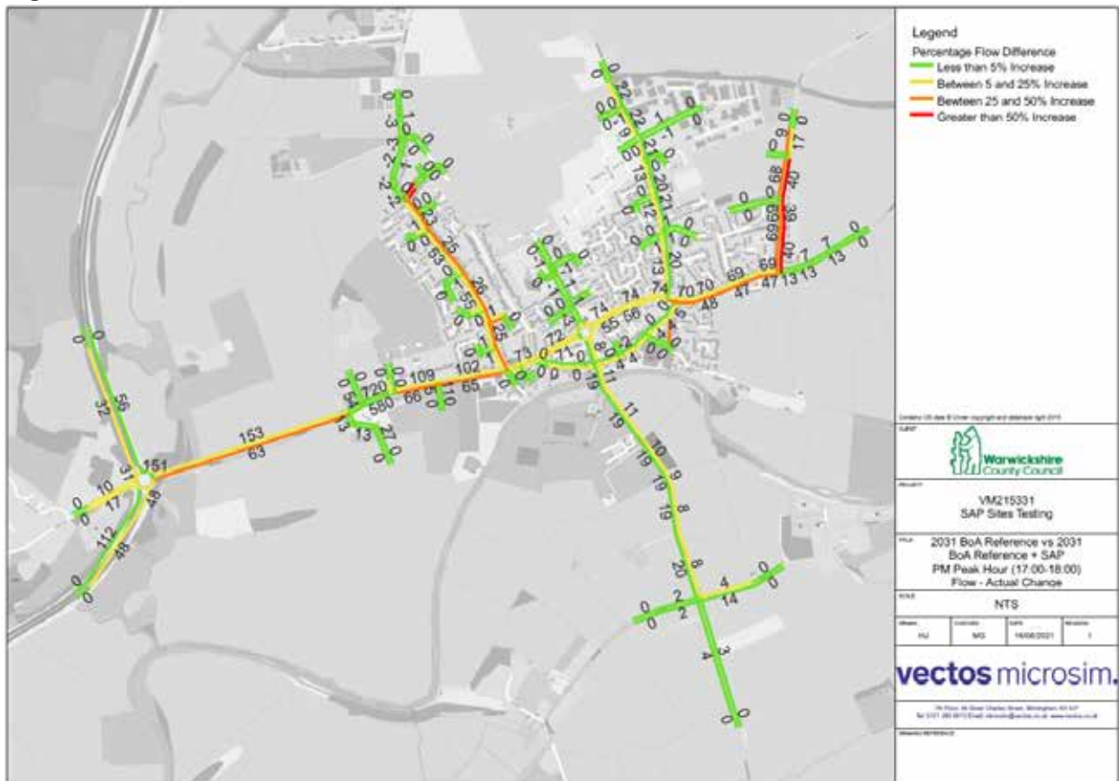
Figure 8 Flow Difference Plot – PM Peak Hour – Reference Case vs Reference + SAP Sites
