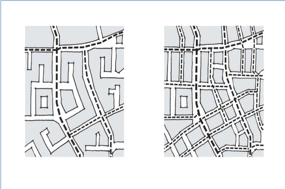
Fig. C.1 - Poor connectivity and good connectivity.
