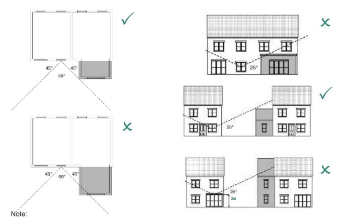
For simplicity, the 25 degree line is measured along the plane of the wall containing the window, as shown.
