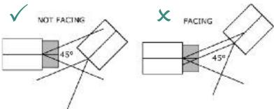
NB: The 45° angle should have equal portions of 22.5° either side of the line that passes through the window at right angles
