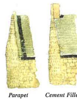
Parapet Cement Fillet
